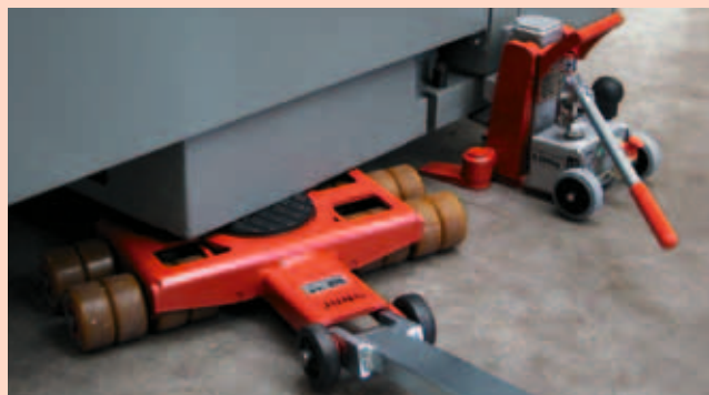
Castors with ball bearings guarantee easy motion
