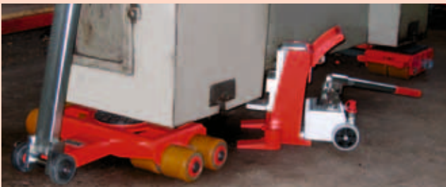
Castors with ball bearings guarantee easy movement
